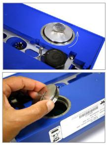
Figure 3: Removing the SIM cover
